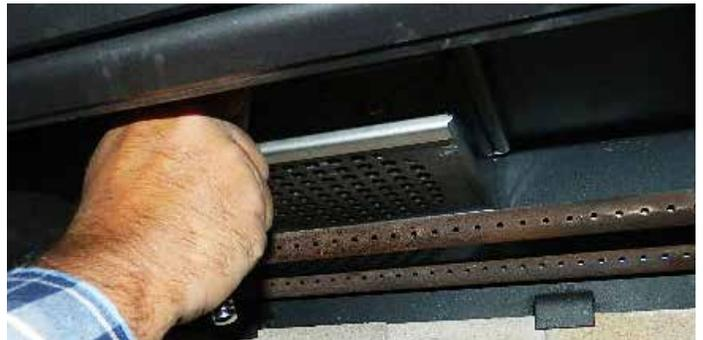
9. Loosen bolts on catalyst retainer then, slide the catalyst retainer to the right to remove.
