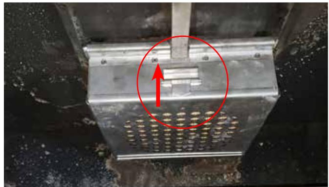
8. Pull the flame shield forward and tilt down, be prepared to support catalyst assembly
