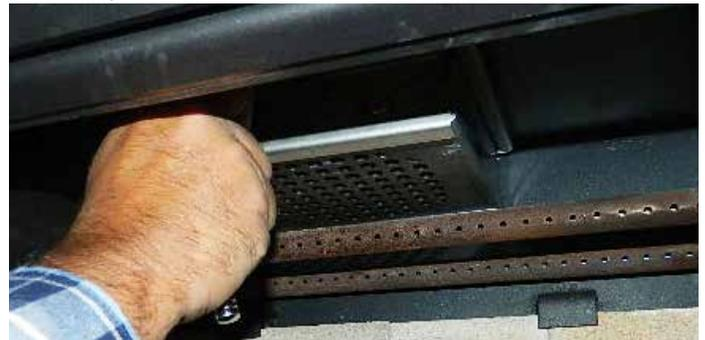
9. Loosen bolts on catalyst retainer, slide the catalyst retainer to the right to remove.
