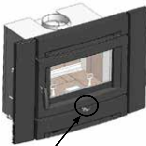
Primary Air Damper Left - Open Right - Closed
