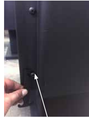
Loosen screw and insert storage bracket.
